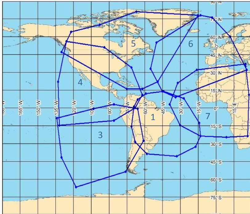
The INMARSAT wide beam footprints shown here were obtained from the Message Type 18 & 19 broadcasts INMARSAT satellite Aero transmissions. These have been overlaid onto an public NGA earth map. available on the web.
